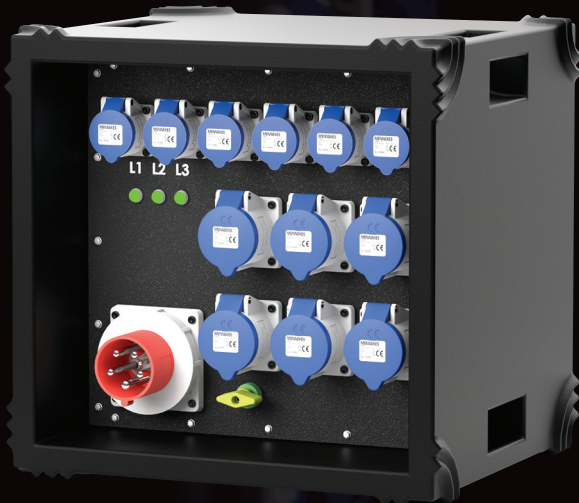
ENC63/415/V45/48/0058/RM 4G Monitoring Distro Inlet: 63A 400V 5PIN Outlet: 6 X 32A 230V 3PIN, 6 X 16A 230V 3PIN
