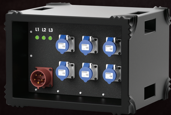
ENC32/415/V45/36/0029/RM 4G Monitoring Distro Inlet: 32A 400V 5 Pin Outlet: 6 x 16A 230V
